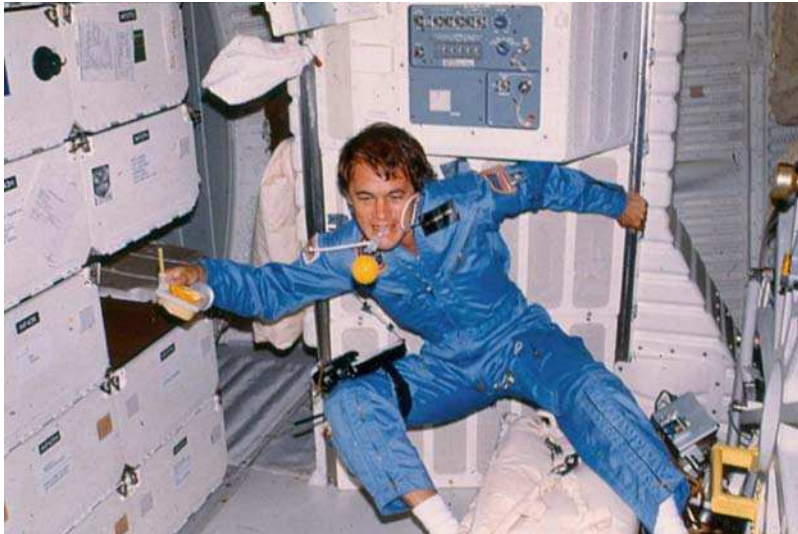
FIGURE 1.6 Astronaut Joe Allen chasing an orange drink on Shuttle. The drink has been squeezed from the package and forms a perfect sphere floating in microgravity (NASA photograph).
